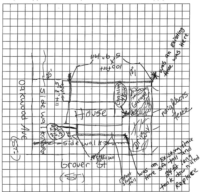
Drawing of proposed fence: Show existing buildings, property lines and easements, location/dimensions of existing fence, if applicable, and location/dimensions of proposed fence. Note: The burden of proof of the exact location of all lot lines shall rest with the property owner.
